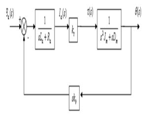
Figure (2): Schematic diagram of the servomotor
