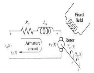
Figure (1): Servomotor system
