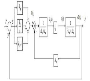
Figure (4): The block diagram of the closed loop servo motor with PID controller.
