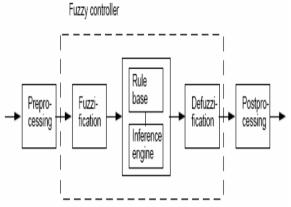
Figure (3):Fuzzy Logic Control Structure
